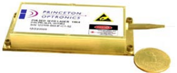
Picture of the seed laser. Package size- 89 x 38 x 15 mm
